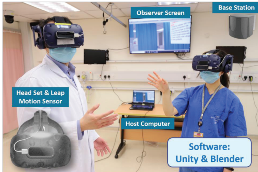
Figure 1: Equipment/setting of virtual reality programme and traditional part-task trainer.
